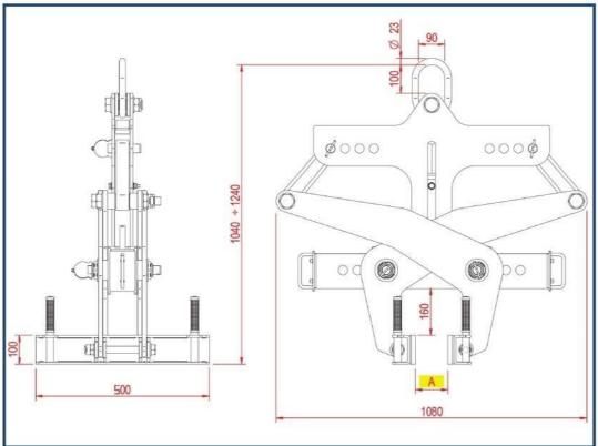
Maximum capacity: 5000 kg. Opening range: O + 400 mm. Surface finish: Zinc plated.
